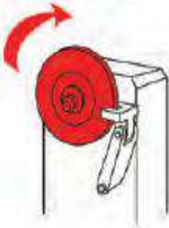
Abrasion and ejection hazard
